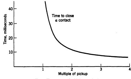
Fig. 2. Time curve of a high-speed relay.
