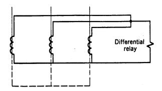
Fig. 17 A three-terminal current-differential application
