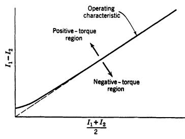
Fig. 19. Operating characteristic of a percentage-differential relay.
