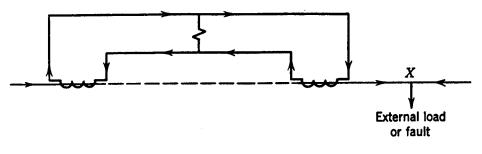
Fig. 15. Conditions for an external load or fault.
