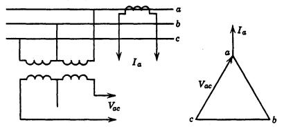
Fig. 5. Connections and vector diagram for a power relay wing phase-to-phase voltage.
