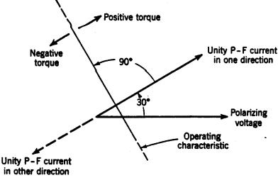
Fig. 7. A typical power-relay operating characteristic.
