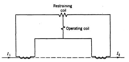
Fig. 18. A percentage-differential relay in a two-terminal circuit.
