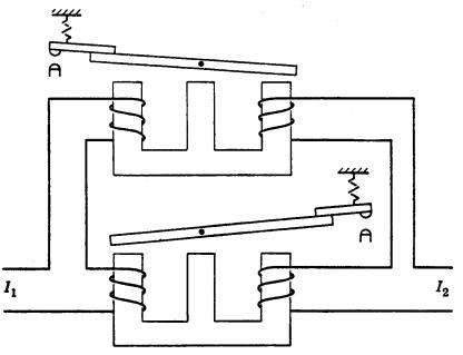
Fig. 11. A two-element current-balance relay
