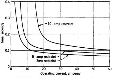
Fig. 12. Time-current curves of a current-balance relay.
