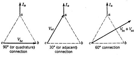
Fig. 8. Conventional connections of directional phase relays.
