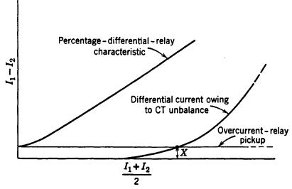
Fig. 20. Illustrating the value of the percentage-differential characteristic.
