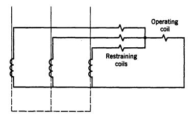
Fig. 21. Three-terminal application of a percentage-differential relay.
