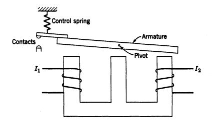
Fig. 9. A balanced-beam type of current-balance relay.
