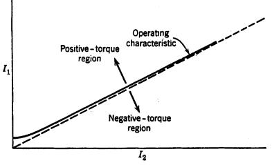
Fig. 10. Operating characteristic of a current-balance relay.
