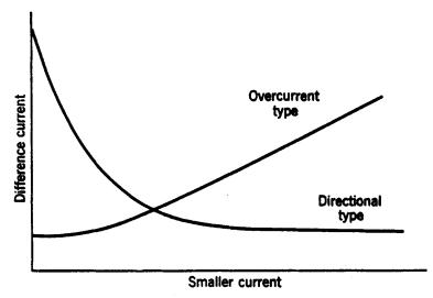
Fig. 13. Comparison of current-balance-relay characteristics.
