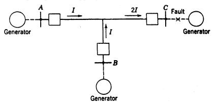
Fig. 4. Illustrating the reduction of sensitivity of phase-comparison relaying on multiterminal lines.
