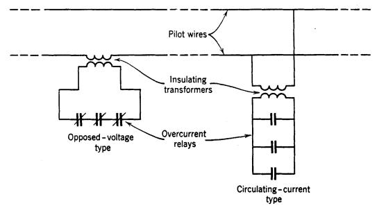
Fig. 2. Blocking-terminal technique.
