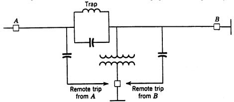
Fig. 6.. Method of avoiding interference by a fault with remote tripping.
