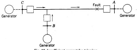
Fig. 10. Insufficient current for tripping.
