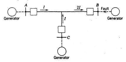
Fig. 11. Directional-comparison blocking relays get twice as much current as tripping relays.
