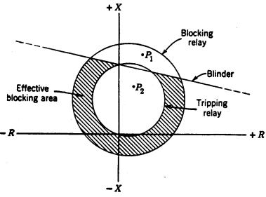
Fig. 14. R-X diagram of the conditions of Fig. 13.
