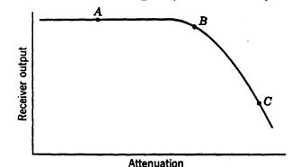
Fig. 3. Effect of attenuation on the strength of the receiver-output signal.
