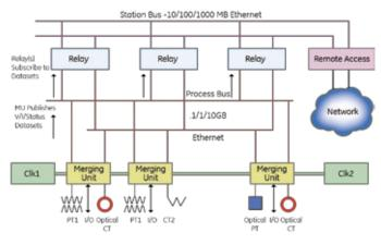
Figure 6. IEC 61850 Substation Model
