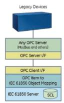
Figure 10. IEC 61850 Data Gateways using OPC
