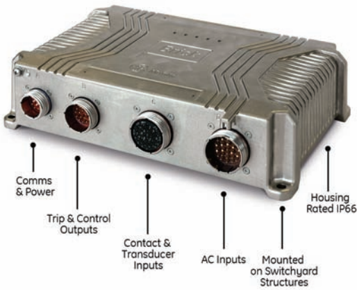
Figure 4. Rugged outdoor merging unit
