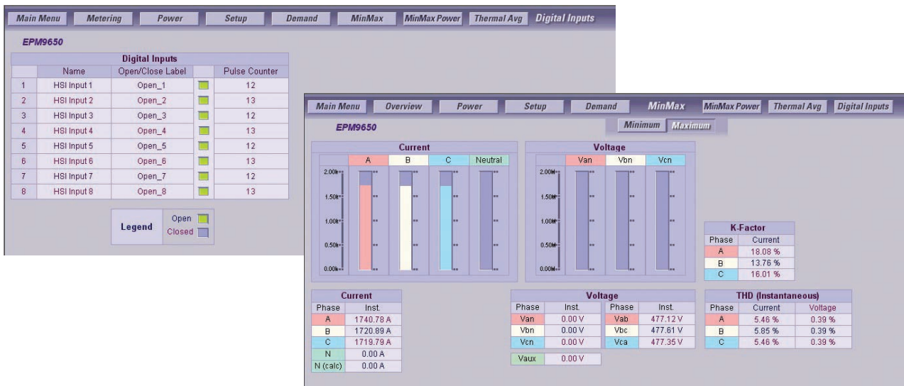
EnerVista Viewpoint Monitoring - Monitor the status of digital inputs and review the magnitude of system highs and lows
